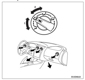
Air flows to the upper part of the passenger compartment and flows to the leg area.
